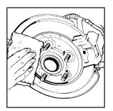
Remove any rust or dirt from the wheel bolts, mounting surfaces, and spare wheel. 11. Install the compact spare tire.
